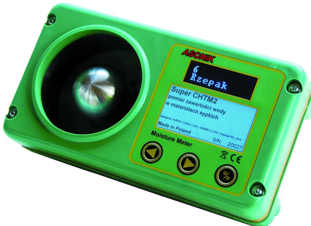
**Super CHTM2 model** is designed to examine the moisture content in many bulky materials, including agricultural substances as well as in further processed materials, chemical and technical materials also. Every unit is programmed with over 100 different calibrations, for example as below:
